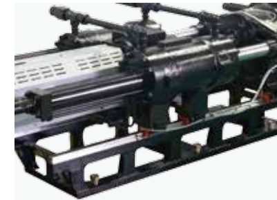
標配線性導軌支座 Injection unit support with linear guide rails
