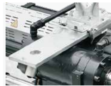
人性化設計：移動料斗滑軌 (320T 及以下) User-friendly design: movable hopper rails (60T-320T)
