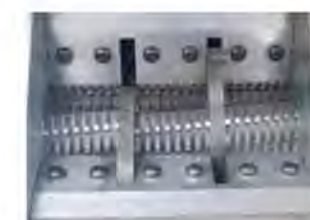
粉碎室 Crushing Room
