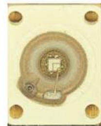
LED with degraded encapsulation
