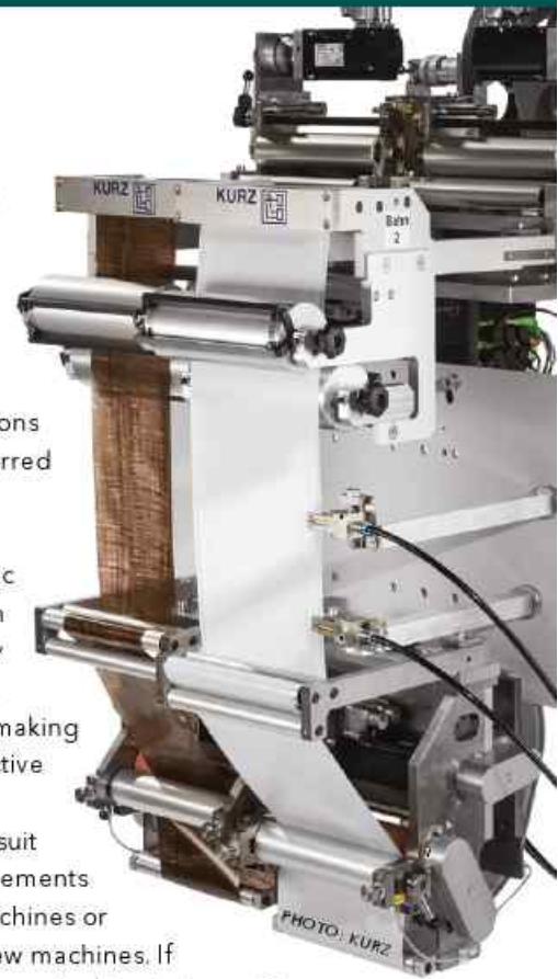
Above: The IMD SI Duo foil feeding unit from Kurz with two precisely positionable foil tracks enables single-image designs to be processed in twin-cavity moulds
