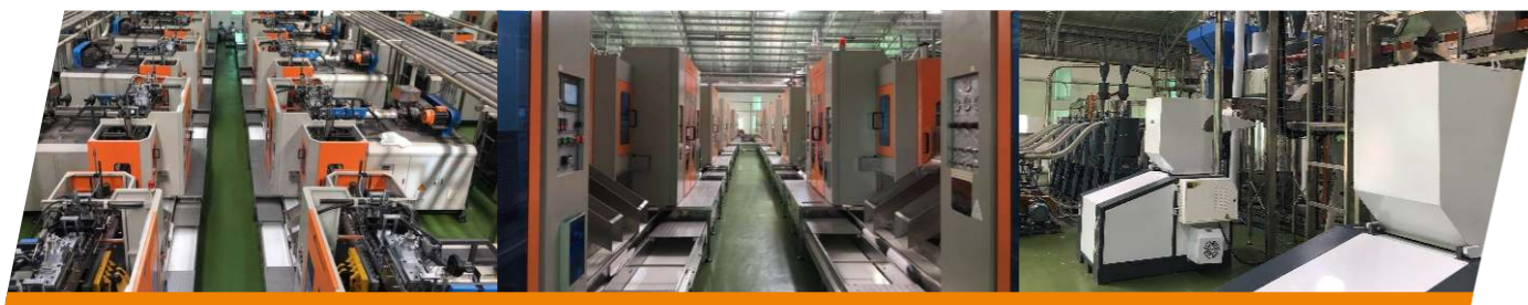
供料、制品输送一体化 Integration of feeding and conveying
